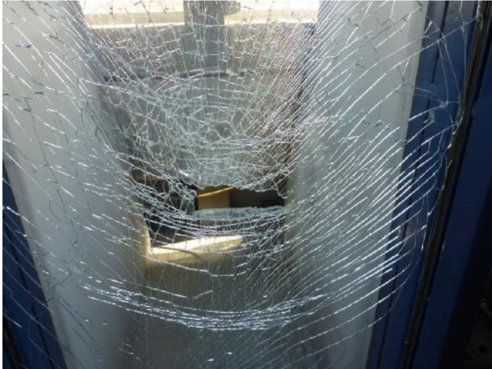
Fig. 2: Sample 2 with breakage behaviour Type B
